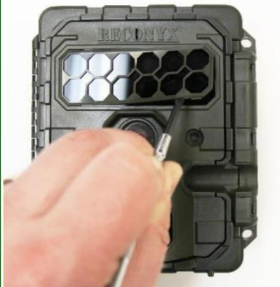
The windows covering the IR Array, lens, WalkTest indicator and light meter may all be cleaned with glass cleaner or water using a soft non-abrasive cloth.
